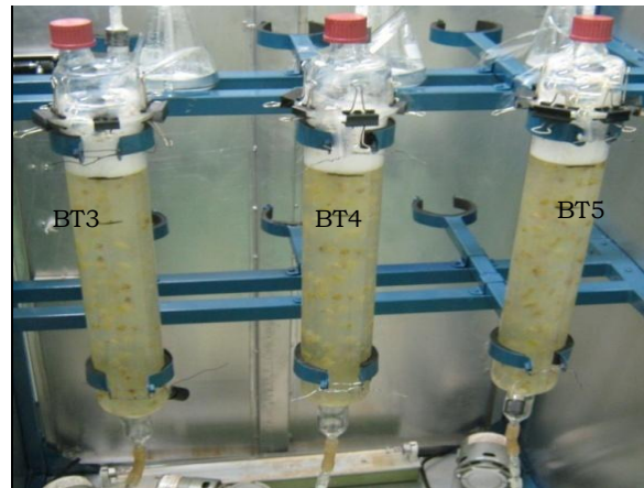
Figure 1. Aggregate cell culture of C.roseus in the bioreactor after 1 day culture in media treatment of the precursor tryptophan. BT3 (150 mg/L), BT4 (200 mg/L) and BT5 (250 mg/L).
