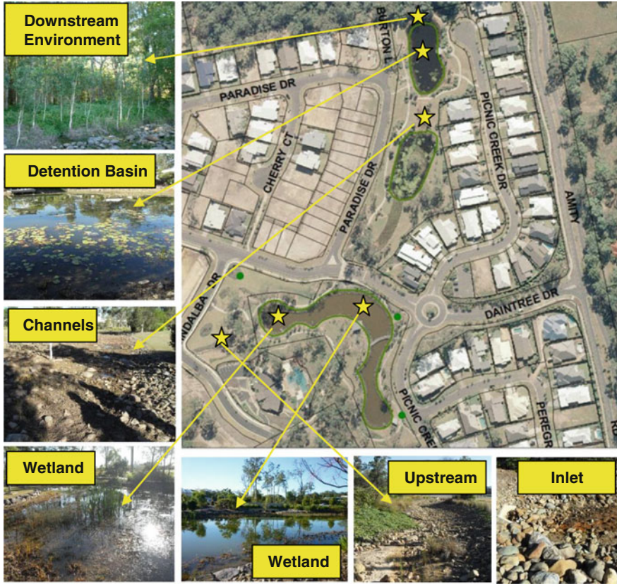
Fig. 1.4 A typical treatment train
