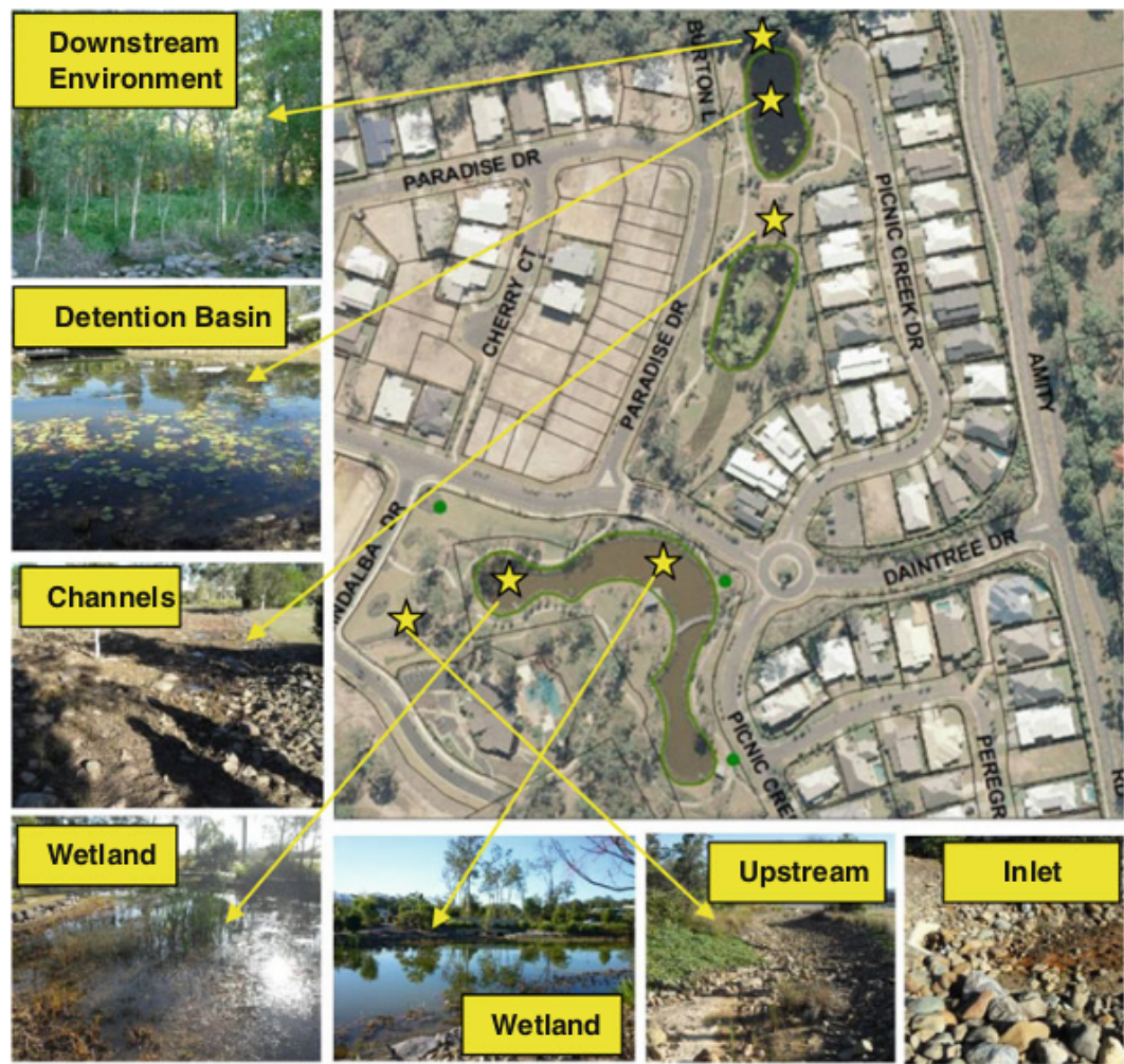
Fig. 1.4 A typical treatment train
