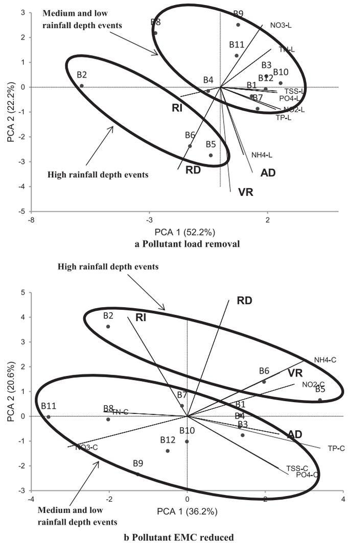
**Fig. 3.** PCA biplot of pollutant removal (AD = antecedent dry period; VR = volume retained; RI = rainfall intensity; RD = rainfall depth; pollutant-L = pollutant load removal percentage; pollutant-C = pollutant EMC reduction percentage).
