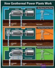
Figure 9 Three of the major types of geothermal power plants.
