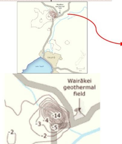
Figure 13. Subsidence around Wairakei Geothermal Field
