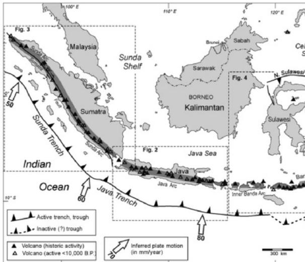
Figure 2 Plate tectonic structures and active volcanic arcs in Indonesia (Hochstein and Sudarman, 2008).
