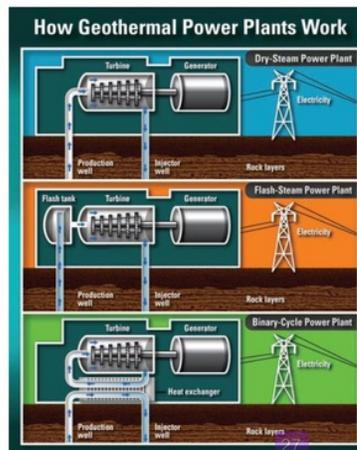
Figure 9 Three of the major types of geothermal power plants.
