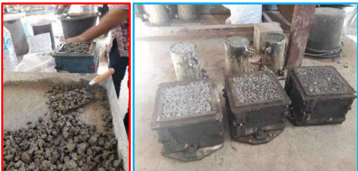
Gambar 7: Sampel-sampel Porous Pavement Beton
