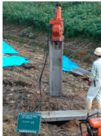
Fig.7 A weighted vibrator is used to penetrate the Geoslicer to the ground.
