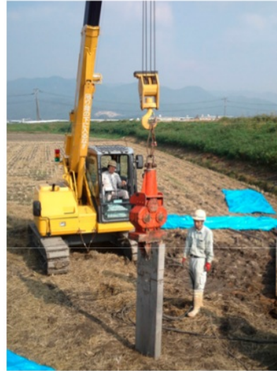
Fig.6 Geotechnical survey using Geoslicer at the retarding basin near No.5 Nokoshi
