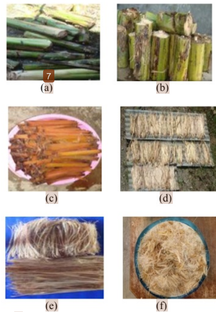
(a) and (b) Banana Trunk, (c) After Boiled, (d) Being Dry in Sun Exposed, (e) Before being cutted, and (f) After be cutted.
