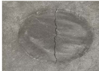
(C) Crack pattern of round panel concrete as tested according to BFT
