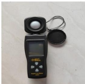
Gambar 2. Alat Ukur Luxmeter
