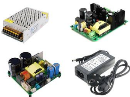
Gambar 6 Power Supply Switching
