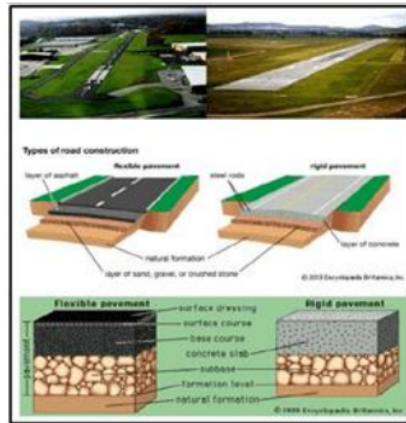
Figure 3. Difference between Rigid Pavement and Flexible Pavement
