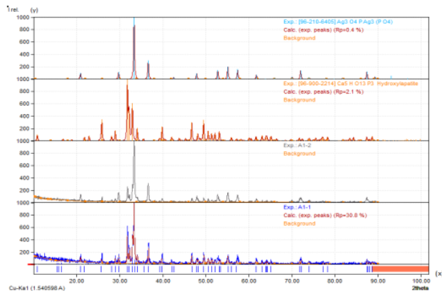
Figure 2. Composite Ag 3 PO 4 /HAp diffractogram at 600°C at the mole ratio of Ag:HAp (5:1 and 2.5:1) with HAp and Ag 3 PO 4 standards
