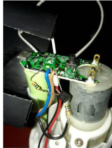
Gambar 7 Gambar Desain Wiring Alat Pompa (Air, Sabun, dan Gel Sanitizer)
