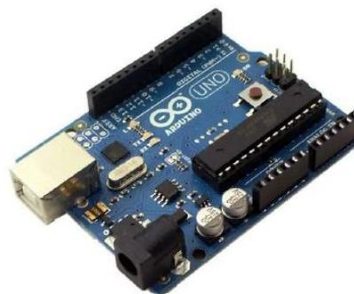
Gambar 1 Board Arduino Uno
