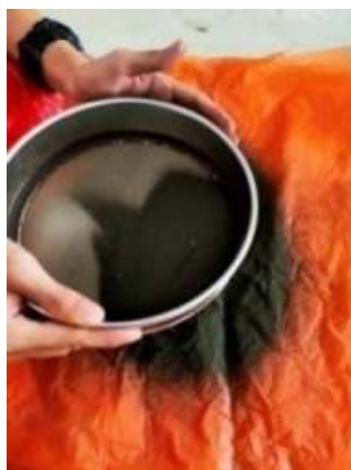
FIGURE 2. The iron sand sieving process uses a 200 mesh sieve.
