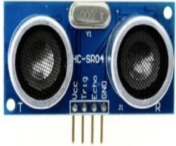
Gambar 4. Sensor Water Level
