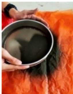
FIGURE 2. The iron sand sieving process uses a 200 mesh sieve.
