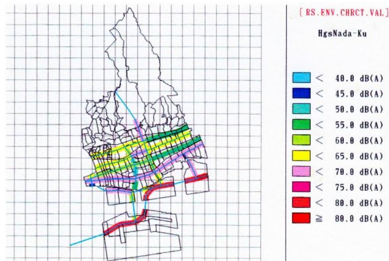
Fig. 10. Display of roadside noise value
