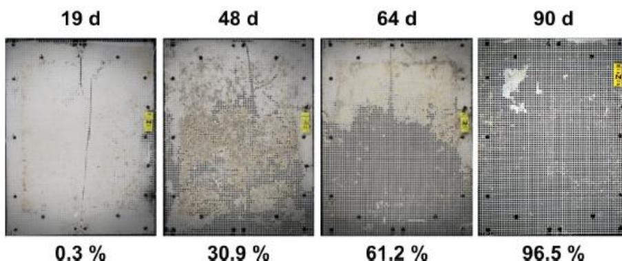
**Fig 8. Exemplary photos of PHA samples from benthic field disintegration tests in SE Asia.** Photos of 1 replicate from 4 exposure intervals each, with disintegration per sample in % area loss below each image. Note: the values are calculated only from the exposed area, not covered by the frame.
