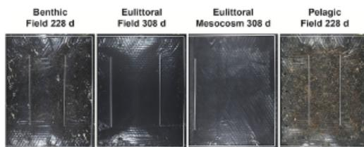
**Fig 7. Exemplary photos of LDPE samples from disintegration tests.** Freshly retrieved samples from field and mesocosm experiments under Mediterranean Sea conditions. Note: the metal bars in the images were put onto the film to keep the sample under water for photography.
