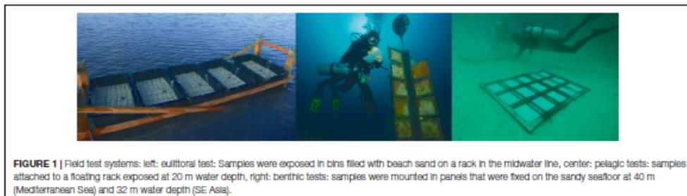
**FIGURE 1** | Field test systems: left: eulittoral test: Samples were exposed in bins filled with beach sand on a rack in the midwater line, center: pelagic tests: samples attached to a floating rack exposed at 20 m water depth, right: benthic tests: samples were mounted in panels that were fixed on the sandy seafloor at 40 m (Mediterranean Sea) and 32 m water depth (SE Asia).
