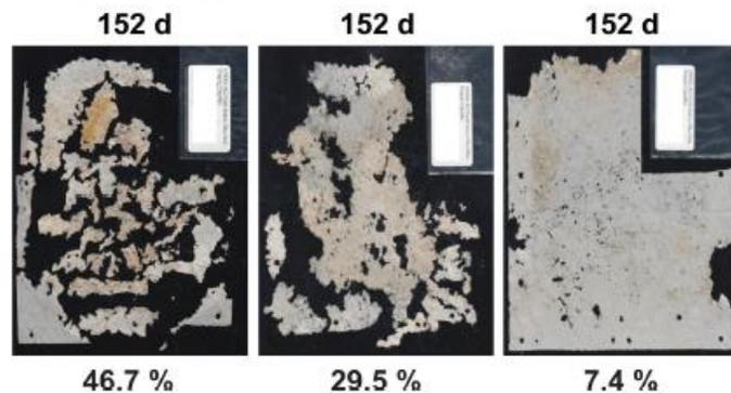
**Fig 10.** Photos of PHA samples from mesocosm benthic disintegration tests to illustrate the heterogeneity between replicates. Scan images of all 3 replicates from the mesocosm benthic test (sublittoral, sea floor scenario) after 152 d of exposure. Disintegration in % are shown below each image. Note the heterogeneous disintegration between the three replicates.
