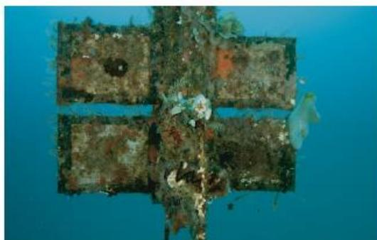
**Fig 12. Fouling at pelagic test system SE Asia at -20 m.** Sample frames and support structure were covered almost completely by sessile animals and algae. Note the fish-size oyster in lower center (zig-zag line). Exposure time 20 months.
