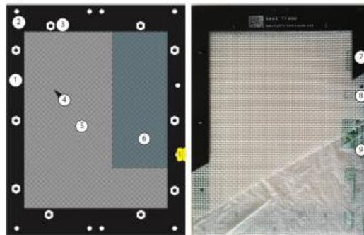
**Fig 1. HYDRA test frame.** Left panel: Scheme of test frame. (1) upper frame, (2) holes for fixing the frame to sample holders, (3) plastic nuts, (4) mesh covering the test material, (5) test material (film), (6) area for subsamples. Right panel: photo of HYDRA test frame, cut open to show different layers. (7) upper frame, (8) upper protective polyester mesh (modified to 2 x 2 mm), (9) test material (plastic bag), seen through film: lower mesh, lower frame.
