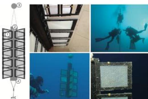
**Fig 4. Pelagic test system.** Left: schematic illustration. (1) test materials in frames with mesh, (2) plastic pipe suspended from a float at 20 m water depth with specimens radially attached, (3) float, (4) steel cable to anchor stone. Upper left: detail of cylindrical rack with specimens attached radially, upper right and lower left: divers at pelagic test system at 20 m water depth. Lower right: detail of specimen in situ, note biofilm after 2 weeks of exposure (Mediterranean Sea).
