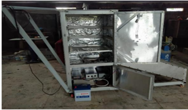
17 FIGURE 3. The result of constructed food dryer integrated with Photovoltaic as the independent power supply
