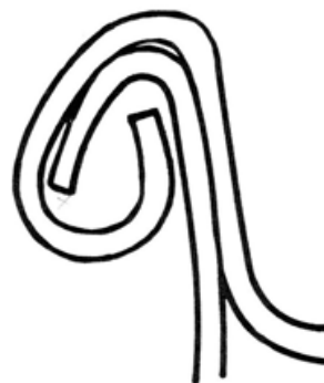
Loose first operation seam.
