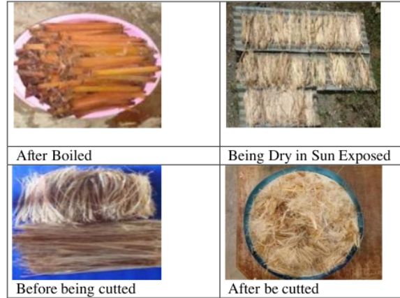
Fig.7. The process of making banana stem fiber.
