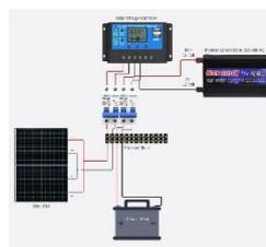
Gambar. 13 Rangkaian Solar Cell, Baterai, Solar Charge Controller, dan Inverter
