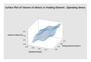
If the operating time is increased, the volume of ethanol will also increase. Additionally, when the operating time is high and the heating element is intensified, the volume of ethanol also iincreases.
