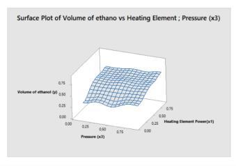
It appears that pressure does not have a significant impact on the volume of ethanol, but what does matter is the heating element power. If the heating element power is increased, whether at low or high pressure, it will affect the volume of ethanol.
