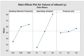
From the above image, it can be observed that the most influential factor on y is x2, which is the operating time.
