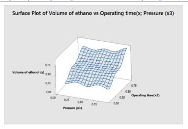
Similarly, it can be concluded that pressure does not have a significant impact on the volume of ethanol, and the most influential factor is the operating time on the volume of ethanol, even at low or high pressure.
